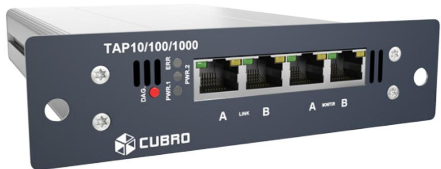
The Cubro 10/100/1000 Copper TAP allows the uninterrupted passage of full duplex data over standard Category 5/6 copper network cable. Featuring auto negotiating between 10Mbps, 100Mbps and 1000Mbps, this TAP duplicates the network signals, including any existing physical errors to the transmit-only monitoring ports.
